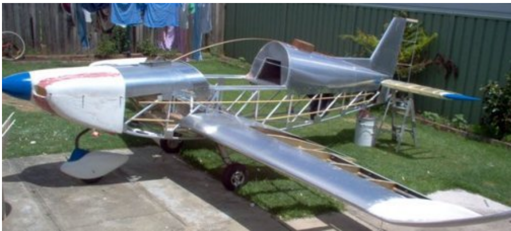
Cheetah prototype uncovered showing construction details..
