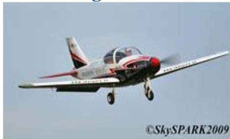
**June 12, 2009** — A new electric-powered aircraft that flew for the first time on Wednesday, June 10, set what's expected to be declared a new world record by flying at a speed of 250 kilometers/hour (155 mph) on Friday, June 12. A specially built Pioneer Alpi 300 - powered by a 75kW electric motor using brushless technology and lithium polymer batteries - made an eight-minute flight at the World Air Games in Turin, Italy, reaching 250 km/hour as a top speed. The SkySpark project, as it is
