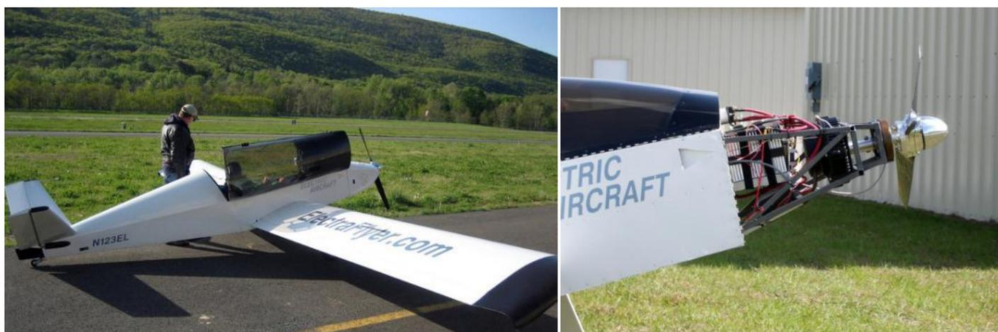
The plane, which has already received its airworthiness certificate, features a 5.6 kWh lithium battery with a projected life cycle (the number of times it can be depleted and recharged) of 1,000 cycles. The battery has a max weight of 78 pounds and can be custom-built to fit the available space in an airplane. It provides juice for a motor driving a 45-inch superlight PowerFin propeller made of a foam core surrounded by an outer shell of carbon fiber and glass fabric.
