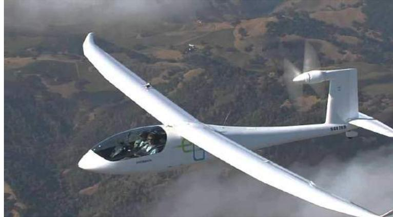
The E-Genius, a 2 seat, electric driven, powered glider
