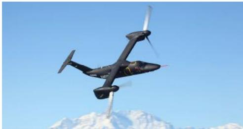
The **AgustaWestland AW609**, formerly the **Bell/AgustaBA609**, is a twin-engined tiltrotor VTOL aircraft with a configuration similar to the Bell Boeing V-22 Osprey. It is capable of landing vertically like a helicopter while having a range and speed in excess of conventional rotorcraft. The AW609 is aimed at the civil aviation market, in particular VIP customers and offshore oil and gas operators.
