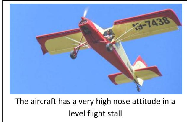
The aircraft has a very high nose attitude in a level flight stall
