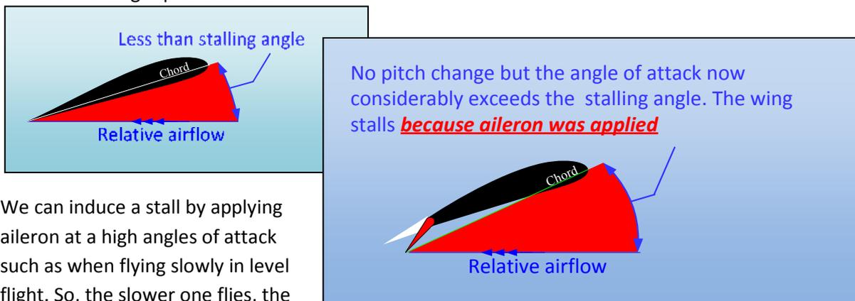
We can induce a stall by applying aileron at a high angles of attack such as when flying slowly in level flight. So, the slower one flies, the more gentle on the controls one needs to be.
