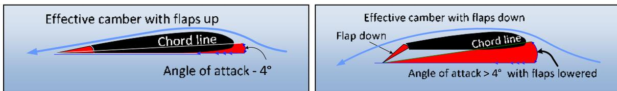
See the sketches above to explain the change in angle of attack when flaps are lowered.
