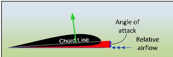
The sketch above depicts the position of the centre of pressure in normal flight. Notice that, in the sketch on the right, the centre of pressure has advanced forward along the chord. It is this advancement with increasing angle of attack that makes
