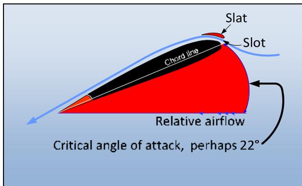
with slot. In truth, the slat is the added physical device, and the slot is the passage created between the device and the aerofoil surface. In other words, slats create slots.
