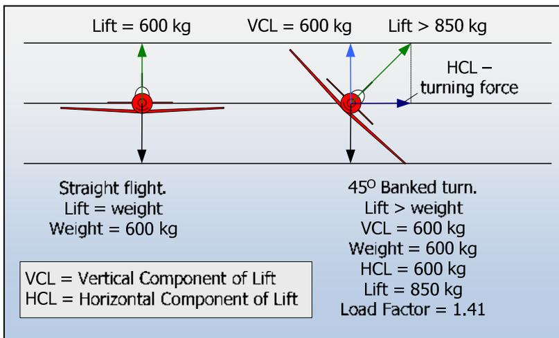
The sketch left is a vector diagram displaying the increasing forces required to turn an aeroplane when it is in balance – i.e. – **NO SLIP OR SKID.**
