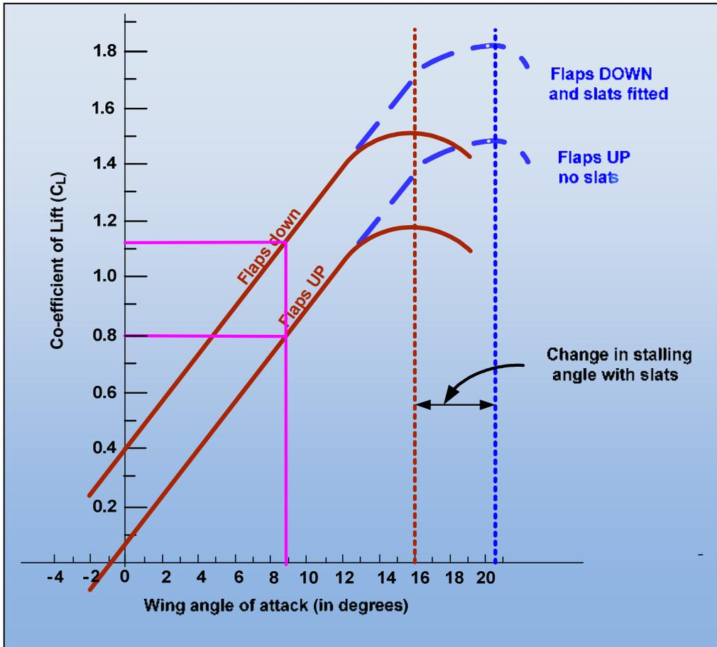
The graph shows that our  $C_L$  value is 0.8 at  $8.8^\circ$  angle of attack with the flaps UP, but notice that this improves to  $C_L$  1.12 at this same angle of attack with the flaps DOWN.
