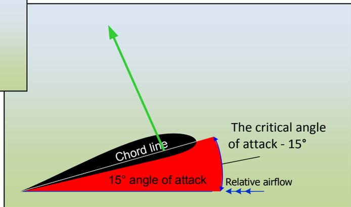
flying with a Centre of Gravity aft of the aeroplane's limits so dangerous. If the angle of attack advances to a point forward of the Centre of Gravity, all the forces acting on the aeroplane will be pitching the nose up and there is no way a pilot can regain control.
