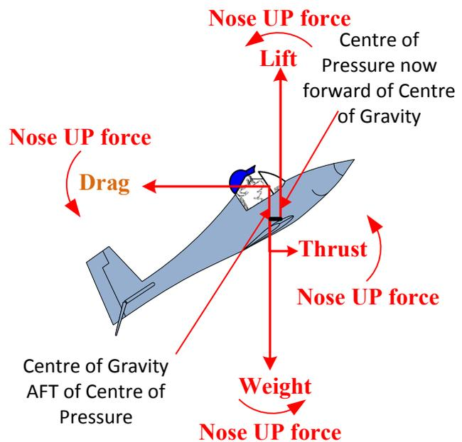
**The Centre of Gravity must ALWAYS be ahead of the Centre of pressure. The aft Centre of Gravity limit must NEVER be exceeded.**
