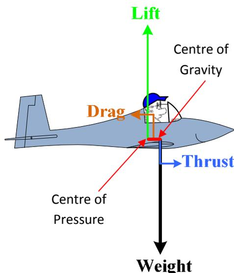
the linear distance between the Centre of Gravity and the Centre of Pressure. And herein lies the problem – as the angle of attack changes so does the location of the Centre of Pressure. With an increase in angle of attack, the Centre of Pressure moves forward along the chord. This is unstable and effectively reduces the arm and thus the strength of the lift/weight couple. This means there is less natural force to hold the nose down and the elevator must be used for attitude control.
