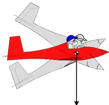
An aeroplane moving about its Centre of Gravity
