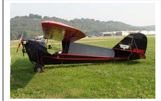
without drag-inducing struts became part of the C-3 design, and the interior was made more elegant with new leather seat cushions. With wheel pants, available as an option since 1931, the two seat light plane attained a top speed of a little over 80 mph despite its low horsepower.
