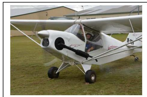
From the test flying surprisingly few changes emerged. A little bit of tweaking perhaps but the only item of note is that I built a set of new and heavier undercarriage frames. Because the machine is short it sits rather nose high. The heavier
