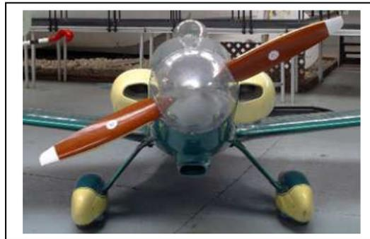
The "Wind". Note the monstrous spinner and the tiny bubble canopy above it.
