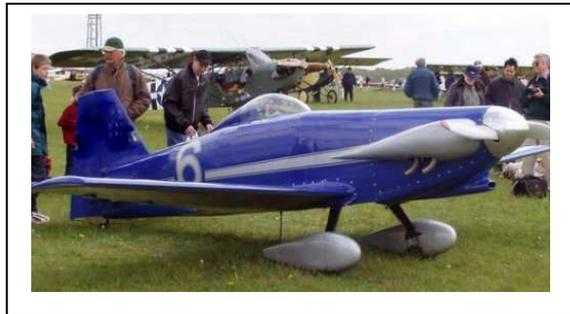
This is a Cosmic Wind. It was designed by Tony Le Vier, the chief test pilot for Lockheed in 1947. Primarily a racer powered by a C-85 (85 hp) hp Continental engine, it was constructed by a group of Lockheed engineers and still flies today in the UK. See the article on page 2 in this publication.
