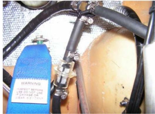
After noting the empty fuel filter, I washed out the fuel lines into white cloth and found nothing. I disassembled the fuel pump and found it in good order.
