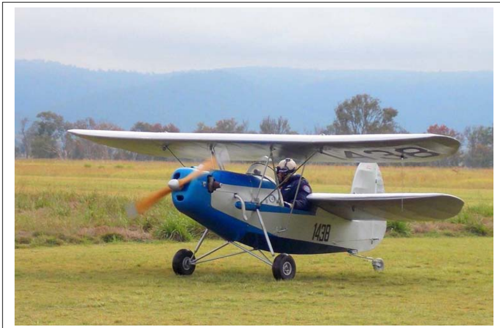
The Pou de Ciel is really a tail-less biplane with super staggered wings.
